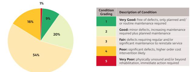
The Torrens Weir is an aging asset, originally constructed in 1881 with sluice gates added in 1929. Majority of its components are rated in a fair to poor condition and engineering inspections and recommendations have identified the need to undertake an options analysis (currently underway) to guide the future management of the asset as it approaches the end of its useful life.
